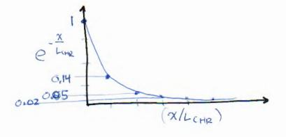
For a fin that is L = 4Lcne or 5 Lcne long, infinitely Long approximation is not so bad! It's bad for this fin, though.
