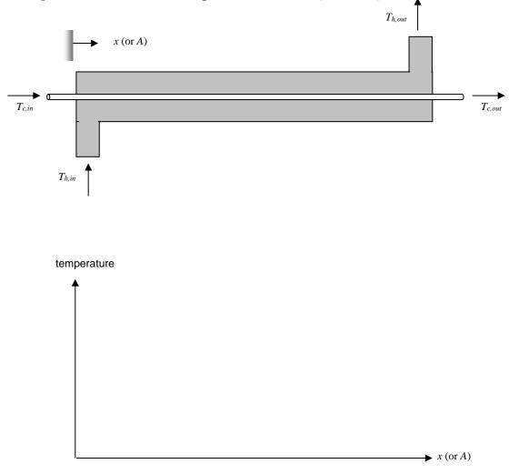
Now consider a *counter-flow* arrangement of the same heat exchanger. The warm fluid inlet temperature is still  $T_{h,in}$  and the cold fluid inlet temperature is still  $T_{c,in}$ . Sketch the variation of fluid temperatures with heat exchanger axial location, x (or area, A).
