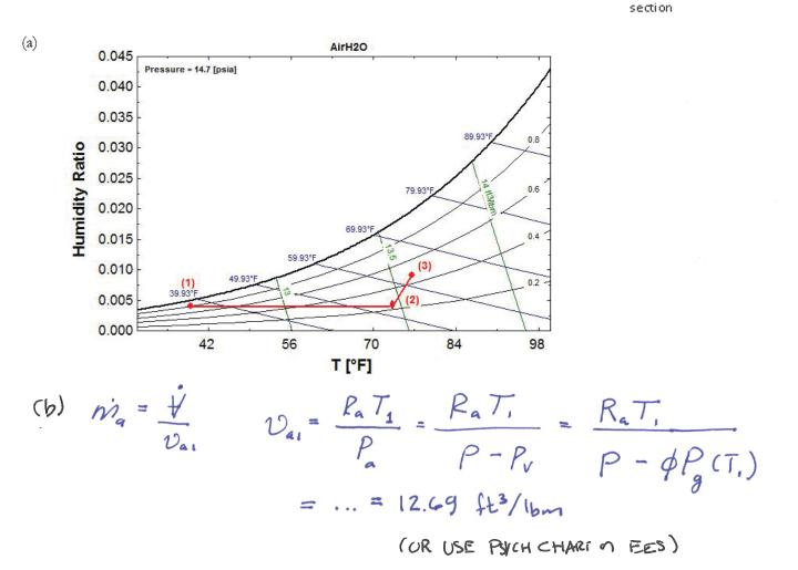
$$\dot{m}_{a} = ... = \frac{2100 \, \text{ft}^{3}/\text{min}}{12.69 \, \text{ft}^{3}/\text{1bm}} = \frac{165.5 \, \text{lbm/min}}{12.69 \, \text{ft}^{3}/\text{1bm}}$$
