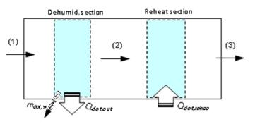
(e) Determine the rate of heat transfer into the air in the reheat section.
