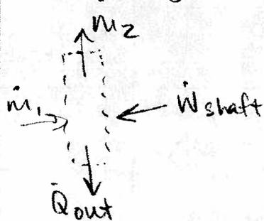
$$\frac{dE_{\text{sys}}}{dt} = \dot{Q}_{\text{in}} + \dot{W} + \dot{m}_1 \left( h_1 + \frac{V_1^2}{2} + g z_1 \right) - \dot{m}_2 \left( h_2 + \frac{V_2^2}{2} + g z_2 \right)$$
