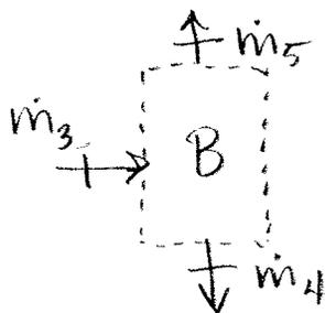
$$\text{Cons Mass } \frac{dm_{\text{sys}}}{dt} = \sum \dot{m}_{\text{in}} - \sum \dot{m}_{\text{out}}$$
