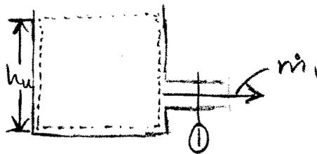
$$\text{Cons Mass: } \frac{dm_{\text{sys}}}{dt} = \sum \dot{m}_{\text{in}} - \sum \dot{m}_{\text{out}}$$
