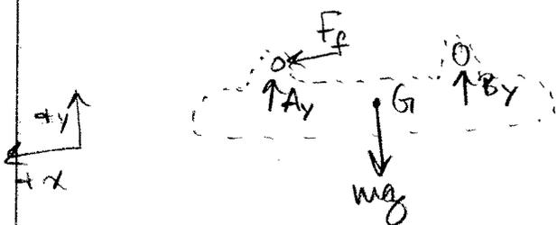
Car moves b/c of  $F_f$  between wheel + track. ... Assume wheels do not slip
