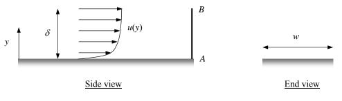
In this region, a fluid speed changes gradually from zero at the wall surface to freestream value ( $u = U_0$ ) at y = d. Assume the velocity profile within the boundary layer is given by
