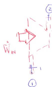
$$0 = \dot{W}_{in} + \dot{m}(h_1 + \frac{V_1^2}{2} + gz_1) - \dot{m}(h_2 + \frac{V_2^2}{2} + gz_2)$$
