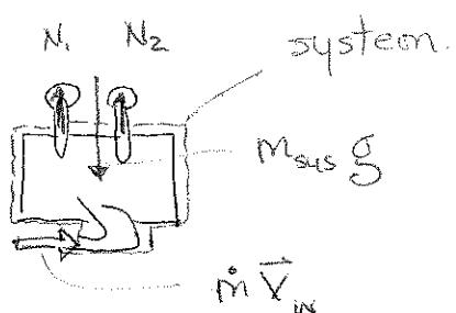
$$\frac{d}{dt}(\vec{P}_{\text{sys}}) = \sum \vec{F} + \sum \dot{m} \vec{v}_{\text{in}} - \sum \dot{m} \vec{v}_{\text{out}}$$
