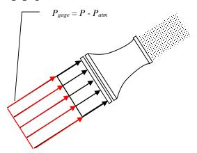
What is the resultant force due to  $P_{atm}$  and the atmospheric component of the inlet pressure?
