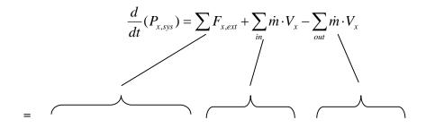
$$R = \dot{m}(V_2 - V_1) - (P_1 - P_{atm})A_1$$
