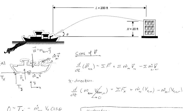
$$0 = T_{\times} - m_{out} V_{o} \cos \theta$$
