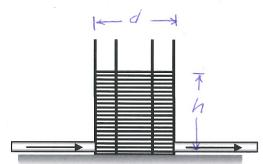
If the tank pressure is uniform and constant and natural gas (methane) can be modeled as an ideal gas with  $R_{\text{methane}}$  =96.3 ft-lbf/lbm-oR, determine the new roof height after the cold snap.
