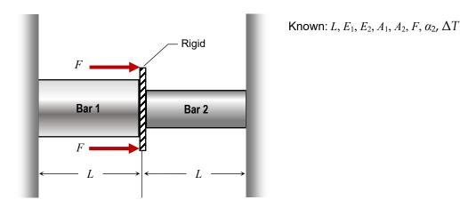
Assuming both bars to be massless, set up the <u>scalar equations that are needed to determine the resulting normal stress in Bar 1</u> after the loading and temperature change. Do not solve the equations but be sure to number the equations and list the unknowns (see the next page).
