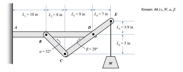
(a) Set up, *but do not solve*, a <u>system of scalar equations necessary to find the reaction(s) at point *A*</u>. Document your solution according to the guidelines established in class.
