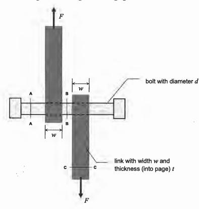
i. [5pts] The shear stress at plane A-A is
