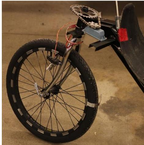
*Figure 6: All-Wheel Steer Prototype*
