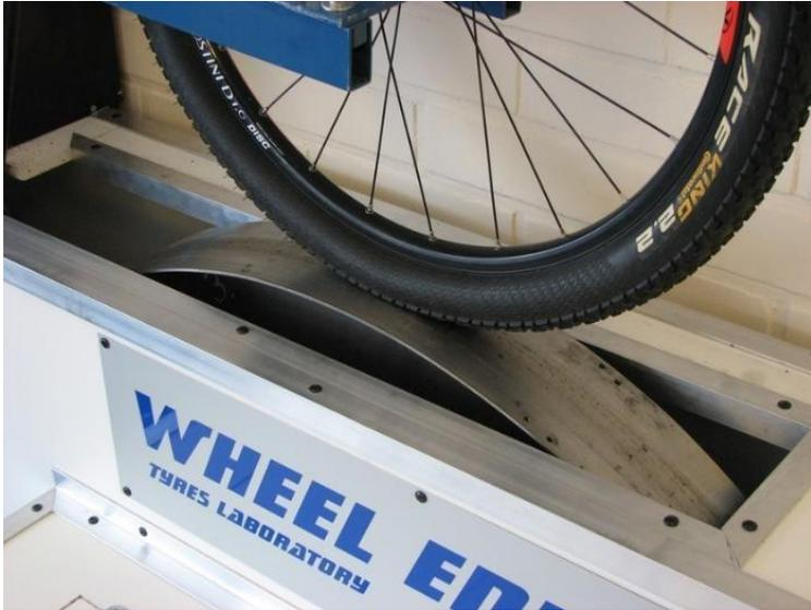
**Figure 8:** Power transfer test with steel drum
