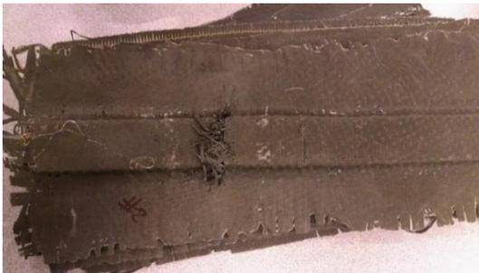
Figure 19. Sample Rib with Epoxy, Chopped Fiber Repair.
