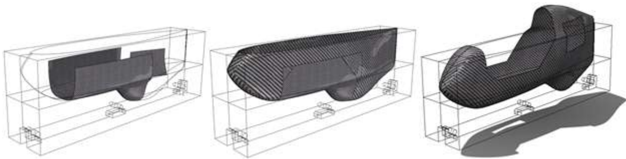
Figure 6: Fairing Layup Steps: Hatches (left), Top Two-Thirds (middle), and Bottom Third (right)
