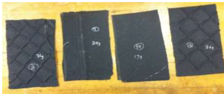
Figure 14: Micro-rib Testing Samples (From left to right: 1 inch square mesh, triangular ¼ inch Nomex rib, flat/control, and 1.5 inch mesh)
