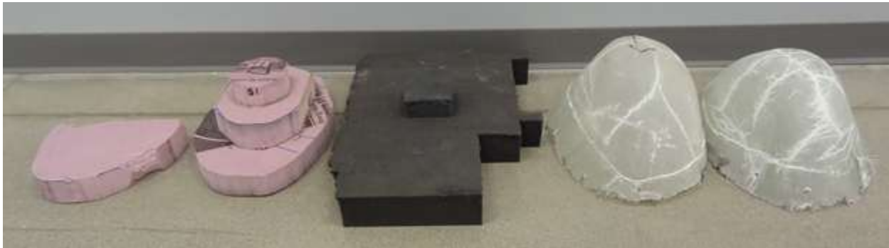
Figure 15: Nose Cone Configurations: Insulation Foam, Cushion Foam, Single and Double Layer Fiberglass
