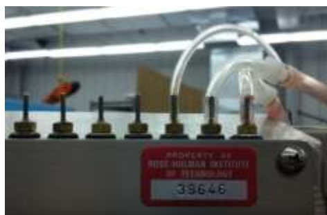
Figure 29: Hookups for the pressure tubes on manometer board
