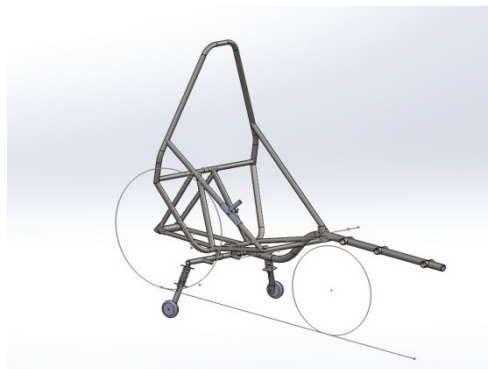
Figure 20: Landing Gear/ Bike Assembly
