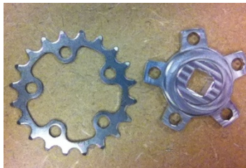
Figure 8: 20-tooth Sprocket with Custom Made Isolated Spider
