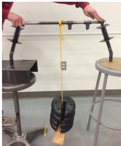
Figure 43: Landing Gear Cyclic Loading Testing
