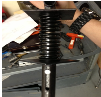
Figure 19: Pin and Slot at Free Height
