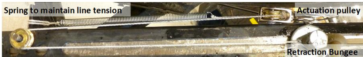
Figure 2: The rider pulls on the actuation cable, causing a pulley to force the innermost tube to extend
