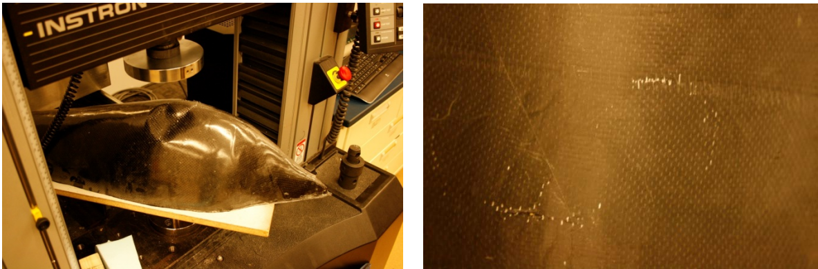
Figure 21:(a) Scale fairing showing deflection, and (b) fractured fiber failure point shown by white streaks.
