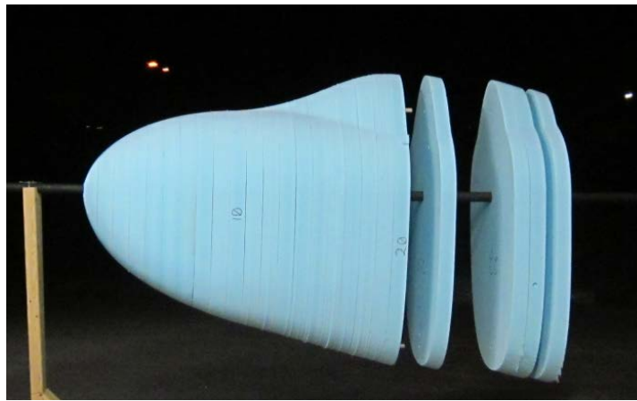
Figure 1: CNC foam pieces forming the male mold. Note that the mold is upside-down in this picture.
