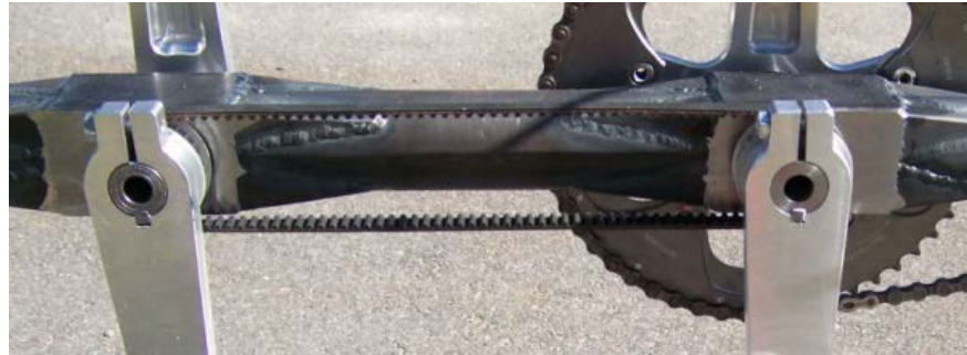
Figure 5: The timing belt mounted to achieve constant forward rotation.
