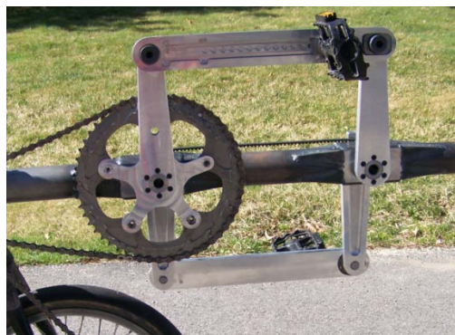
Figure 4: The rider compensation system mounted on Charlie, our current prototype.
