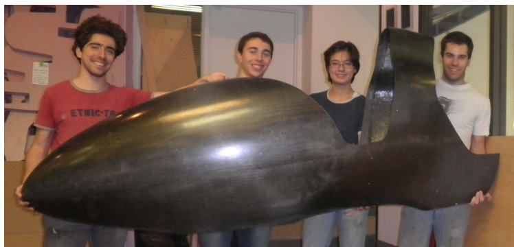
Figure 1: Current status of construction, with monocoque shell complete.
