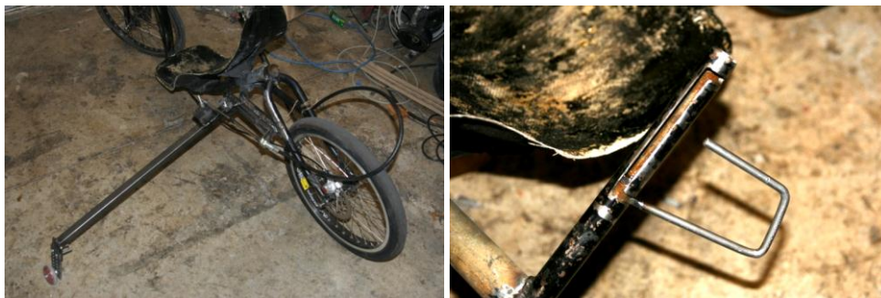
Figure 2: Landing Gear Prototype with Latch Mechanism
