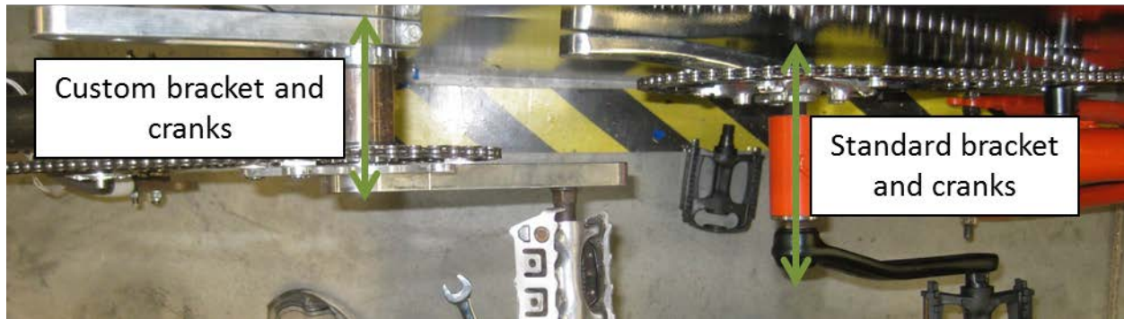
Figure 5: Custom Crank Comparison. Note custom narrower bracket and custom flat cranks on the prototype vehicle to the left. These changes narrow the footpath by 2.75in.
