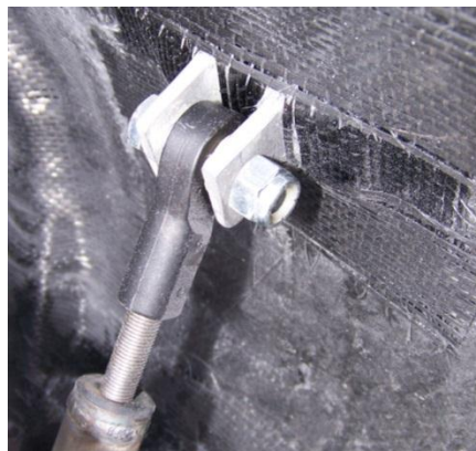
Figure 4: Fairing Attachment Method. Out of picture, the tie rod and tube are bolted to the frame.
