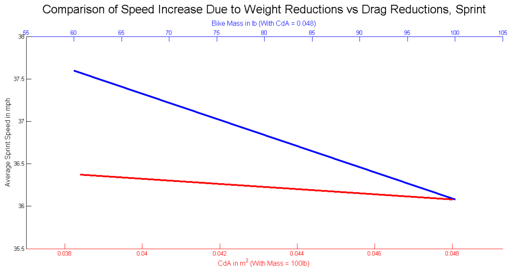
Figure 20: Comparison of Speed with Respect to Weight and Drag Reductions (Sprint). The average speed during the sprint race is significantly affected by vehicle mass, but not by the C_dA .
