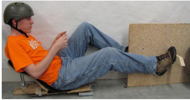
Figure 7: Rider Measurement. From this setup we were able to make a complete rider profile on which to base our fairing shape.
