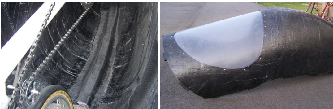
Figure 3: a) Rib on Bottom of Fairing. b) Canopy Section with Pop-Riveted Window
