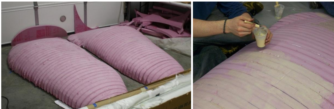
Figure 2: a) Left and Right Mold Halves. b) Applying diluted wood glue to half of the fairing mold.
