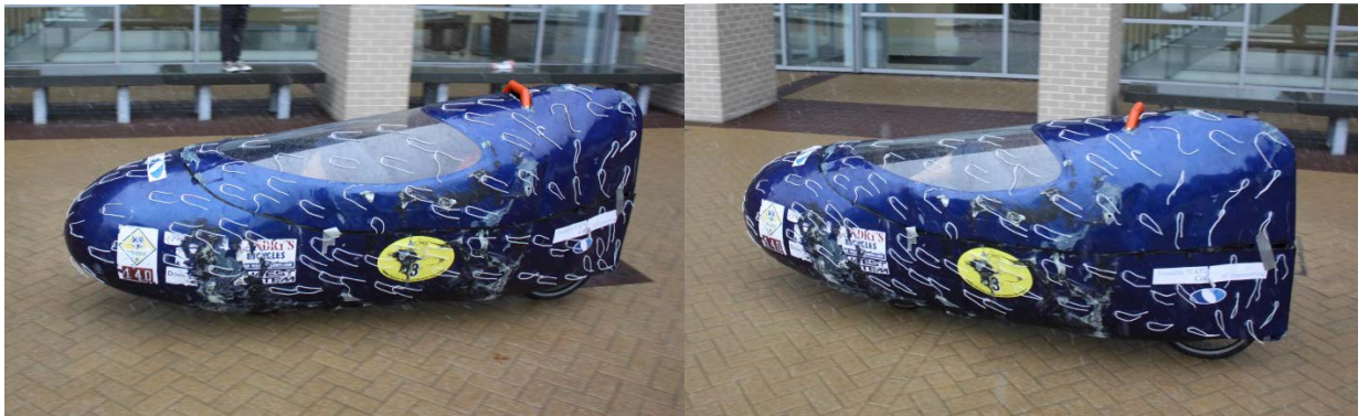
Figure 25: Yarn Tuft Testing. The disturbances in the white yarn show the flow over the fairing surface.
