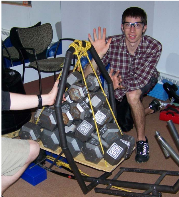
Figure 27: Vertical load testing. 600lbf was suspended 12° from vertical. The roll bar successfully passed the loading test and only displaced elastically under load. The team members pictured are applying negligible horizontal forces to balance the vehicle.
