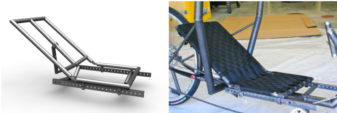
Figure 3: CAD Seat Model and Manufactured Seat. The triangular linkage system on the seat back provides an adjustable seat angle and rails allow for positional changes. A hammock woven across the steel frame to provides the rider a lightweight seat. The weaving is backed with foam padding for added comfort.
