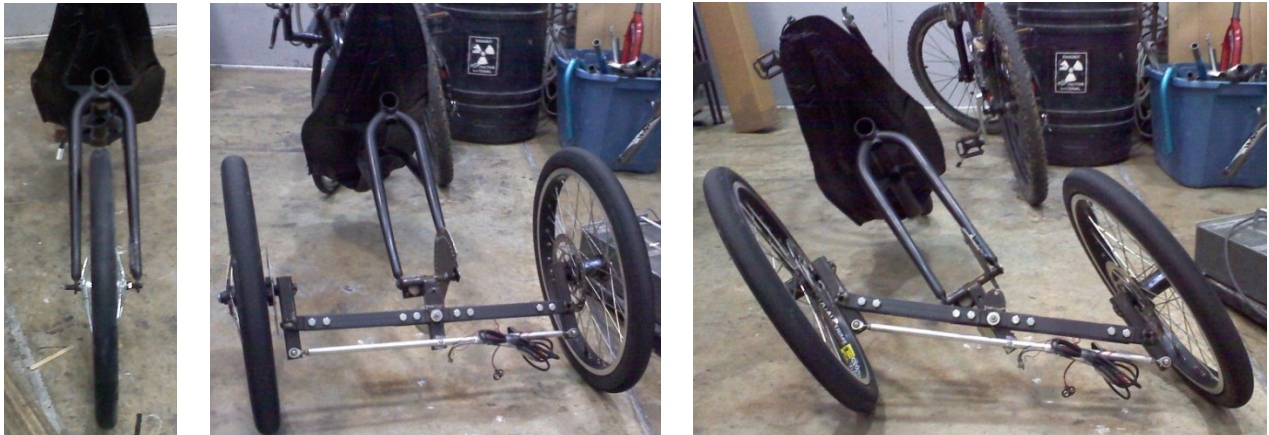
Figure 2: Prototype of interchangeable tilting trike assembly
