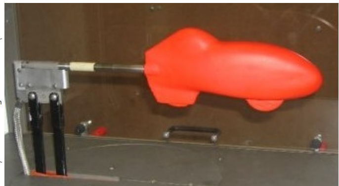
Figure 19: Sting Balance Testing Setup
