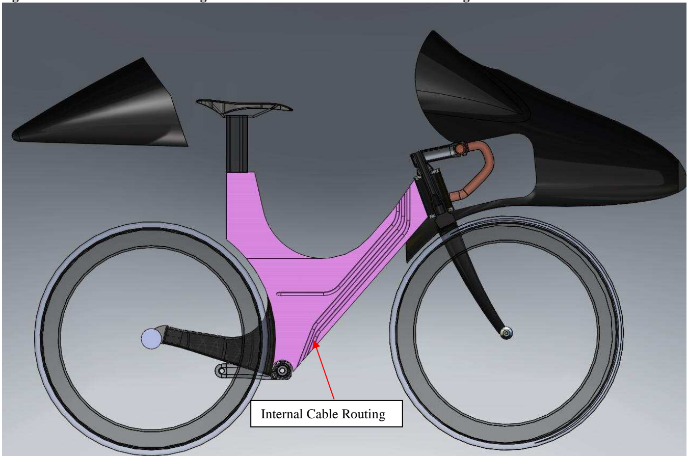
Figure 7. Cross Section Illustrating Pink Foam Core and Internal Cable Routing
