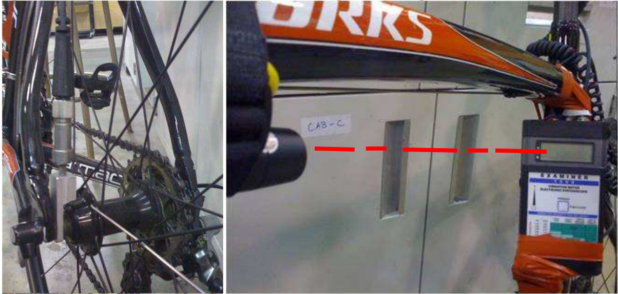
Figure 15. Accelerometer Road Test Fixture and Data Acquisition Set Up
