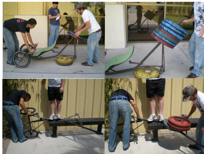
Figure 40: Roll bar Load Testing
