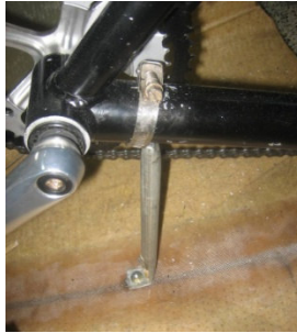
Figure 41: Support Rod Testing
