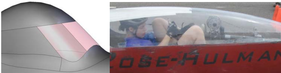
Figure 11 – (Left) The Infinity will have a flat sheet of plastic in a 2-d bend (Right) Long gradual canopies have great side visibility, but are hard to see forward through such a shallow angle.
