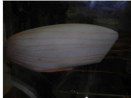
Figure 4.1b Flow string test
