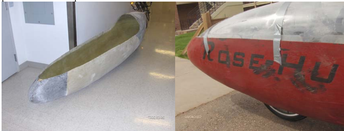
Figure 16: The picture on the left is of the fairing before it was painted. The yellow patch is the extra Kevlar. The picture on the right is of the fairing after a crash on asphalt. The scratches on the paint line up with where the patch was placed.
