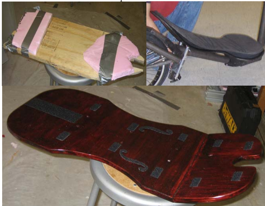
Figure 6: Evolution of Seat Design. Top Left - First Seat Top Right - Donated Carbon Fiber Seat Bottom - Final Wood and Foam Seat
