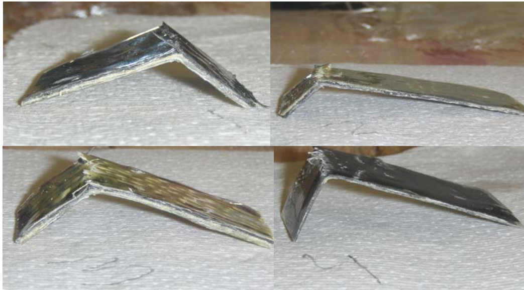
Figure 15: The top-left picture is of sample 1. Note the long shard at the break. This failure mode disqualified this arrangement. The top-right picture is of sample 2. The surface is fuzzy after the break with several blunt shards. The bottom-left picture is of sample 3. There is little fuzz, and more shards than sample 2. The bottom-right picture is of sample 4. There are two or three blunt shards at the break.
