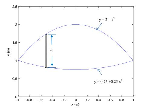
The equation for the y-centroid of the shape may be written (using a vertical strip) as
