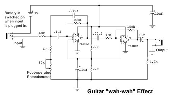
This is essentially a low-Q bandpass filter with the cutoff frequency determined by a potientiometer. By placing the pot in a foot-operatred pedal, guitarists can use the "wah-wah" effect for expression.
