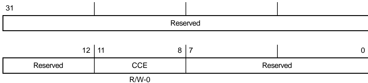
Figure B–43. EDMA Channel Chain Enable Register (CCER)
