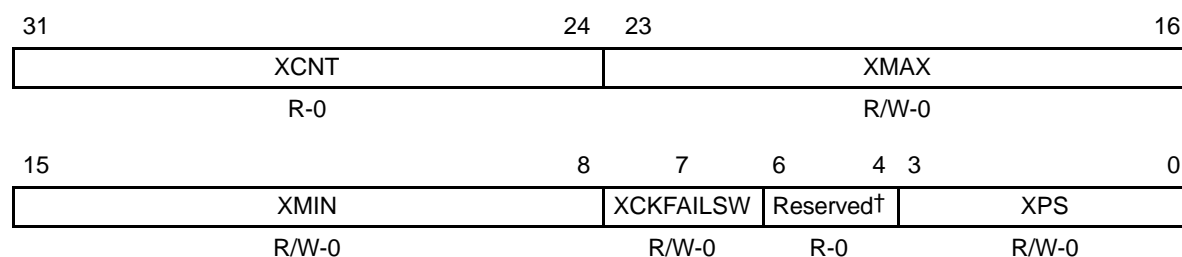
Figure B–146. Transmit Clock Check Control Register (XCLKCHK) [Offset 00C8h]
