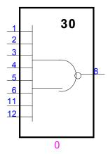
2 (Decoder) Implement a two-bit subtractor with borrow using 74LS138 decoder chips and either 74LS20 or 74LS30 chips as needed. The subtractor has two 2-bit inputs A1A0 and B1B0. It has three bit output, D1, D0 and Borrow. D1D0 = A1A0-B1B0 and Borrow when A1A0 is less than B1B0.
