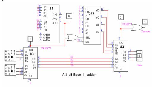
Here is my device test schematic:
