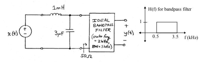
Find y(t). Note: The bandpass filter looks like a 50  $\Omega$  resistor to the inductor/capacitor portion of the circuit.
