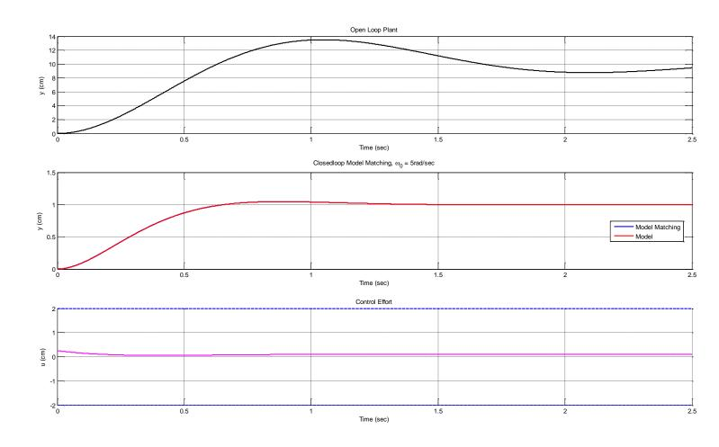
Figure 4. Response of a plant and an ITAE closed loop model matching system.
