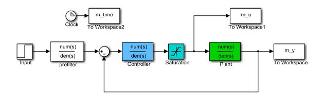
Figure 3. Simple feedback control system
