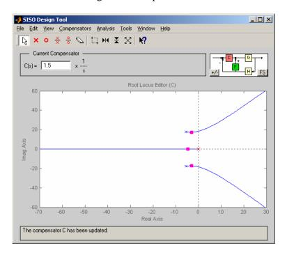
Note that this looks like the root locus plot for an I controller! The step response for this configuration is shown below. Note that the control effort is very small at the initial time. If the step response is not acceptable, first try modifying C(s) then F(s).
