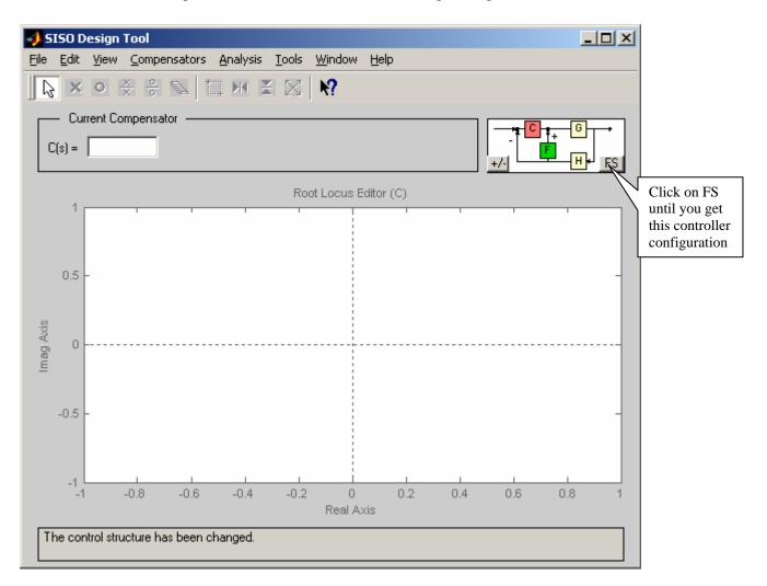
Sisotool will allow us to modify both C(s) and F(s), but it is much easier to modify C(s). We will have to iterate between both of these.
