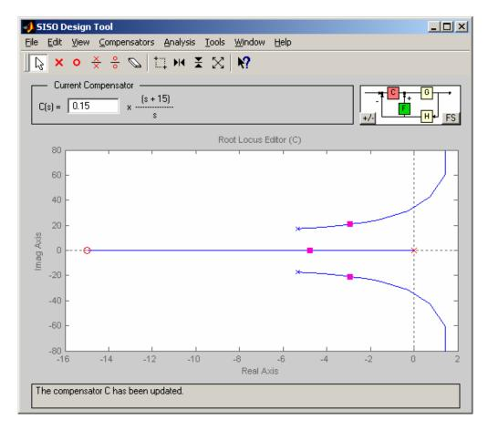
Here we can see the pole at the origin and the zero at -15 due to C(s). This looks like the root locus plot for a PI controller. At this point we can drag the zero around and also drag the red squares around (which change the gain value). However, we can do nothing to change F(s) except to edit it.
