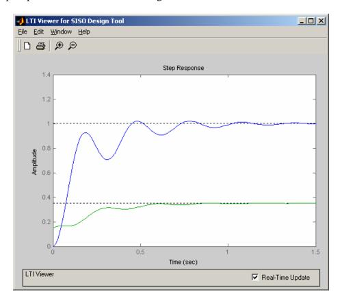
Note that, compared to a normal PID controller, the control effort is not infinite at 0, and actually builds as time goes on (like an integral controller). At this point we might want to go back modify C(s) to see if we get acceptable performance. If we cannot get acceptable performance we may then have to try another value for F(s).
