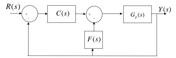
show that the transfer function from input to output is given by
