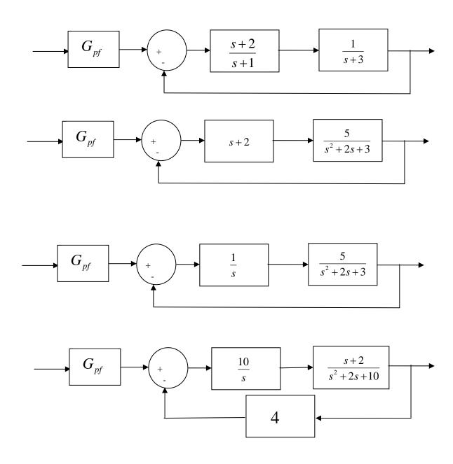
4) For the following system, with prefilter  $G_{pf}$ , plant  $G_p(s) = \frac{1}{s+1}$ , and controller  $G_c(s)$
