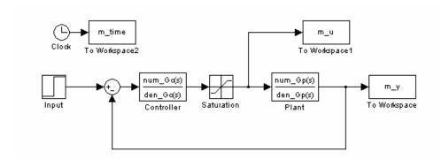
This is a <u>closed loop</u> system, in that we are feeding back the output and comparing this output to what we wanted the output to be. We have also added a new transfer function, the *controller* or *compensator*, usually denoted as Gc(s).
