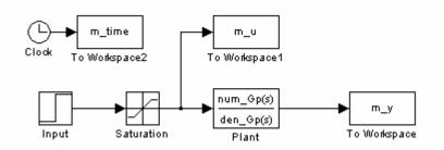
In this case, all of the things we are saving (to plot later) have the prefix m, such as  $m\_time$ ,  $m\_u$ , and  $m\_y$ . This is so we can (in future labs) compare the response of the model (the m things) with the response of the real system.
