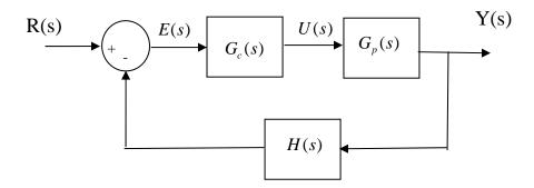
The (closed loop) transfer function between the input and output is given by
