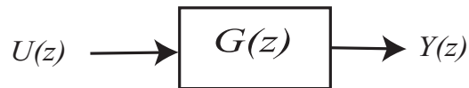
Figure 64: Discrete-time transfer function, G(z) = \frac{Y(z)}{U(z)} . Discrete-time transfer functions are often implemented in terms of the difference equation they represent.
