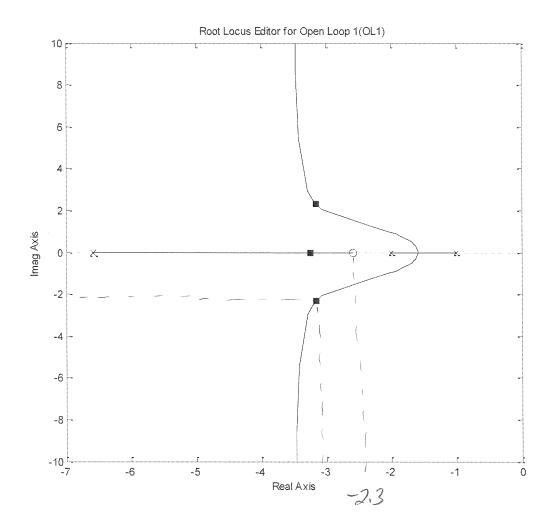
11) When k = 14.1 the poles are as they are shown in the figure. Estimate the closed loop poles.
