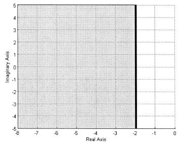
18) One of the shaded regions below shows the possible pole locations for a percent overshoot less than 10%, and the other shows the possible pole locations for a percent overshoot less than 20%. Which of the two graphs shows the possible pole locations for a percent overshoot less than 20%?
