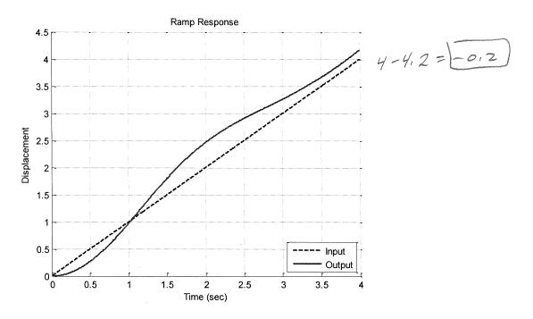
5) Estimate the steady state error for the ramp response of the system shown below:
