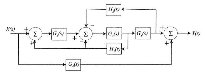
a) Draw the corresponding signal flow graph, labeling each branch and direction
