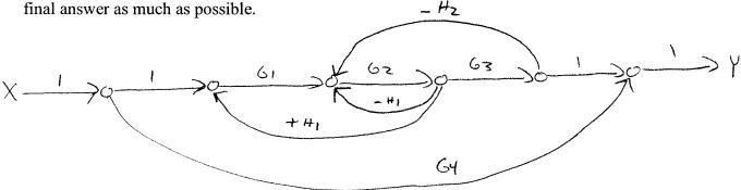
$$P_{1} = G_{1}G_{2}G_{3} \qquad P_{2} = G_{4} \qquad L_{1} = -G_{2}G_{3}H_{2} \qquad L_{2} = -H_{1}G_{2} \qquad L_{3} = G_{1}b_{2}H_{1}$$
