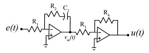
Determine expression for both  $k_p$  and  $k_i$  in terms of the parameters  $R_1, R_2, R_3, R_4, C_2$
