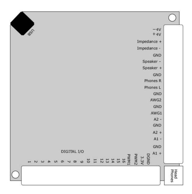
Connect the source (**AWG1**) and ground (**GND**) as the input to your circuit, and connect **A1**+ to the positive end of the capacitor (where you think it will be positive) and connect **A1**- to the negative end of the capacitor. If you get these reversed you will just get an output that is the negative of what you expect.
