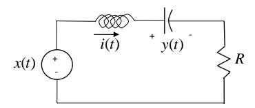
For this circuit, use your variable resistor for R, use a 0.01  $\mu$  fcapacitor, and a 33 mH inductor. <u>You will need to get the inductor from me.</u>
