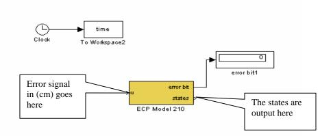
The next step is to remove the model of the system and the output from your Simulink model of the system, and merge the two Simulink files
