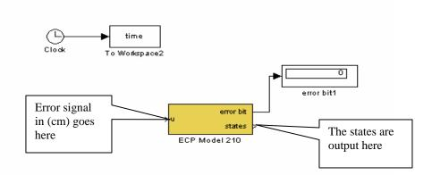
The next step is to remove the model of the system and the output from your Simulink model of the system, and prepare to merge the two Simulink files
