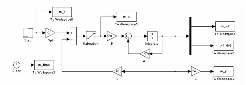
All of the output variable names begin with an m, such as  $\underline{\mathbf{m}} \times \mathbf{1}$ . This is to distinguish the variables from the model with the actual values from the ECP system.
