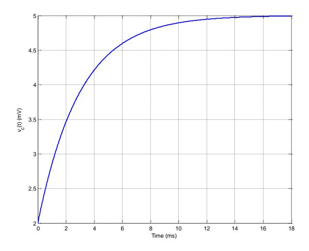
Based on this figure, the best estimate of the **time constant** for this system is
