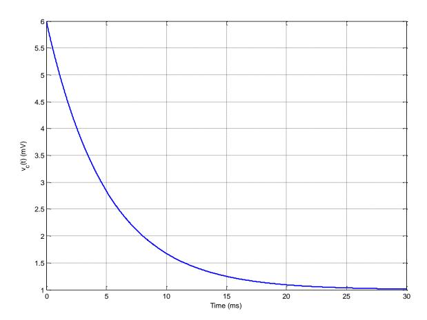
Based on this figure, the best estimate of the **time constant** for this system is
