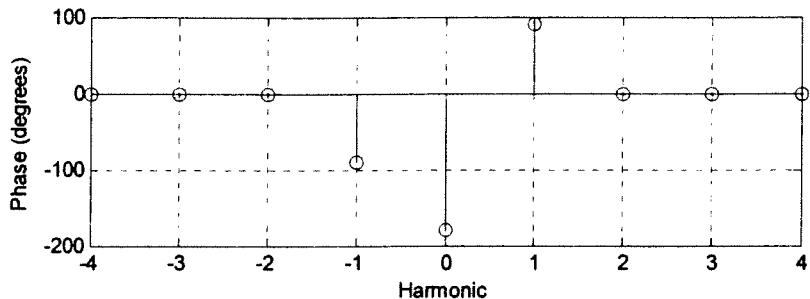
The system transfer function,  $H(k\omega_0)$ , has the following spectrum:
