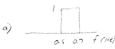
remove all signals with frequencies outside 0.5 to 0.7 Hz
