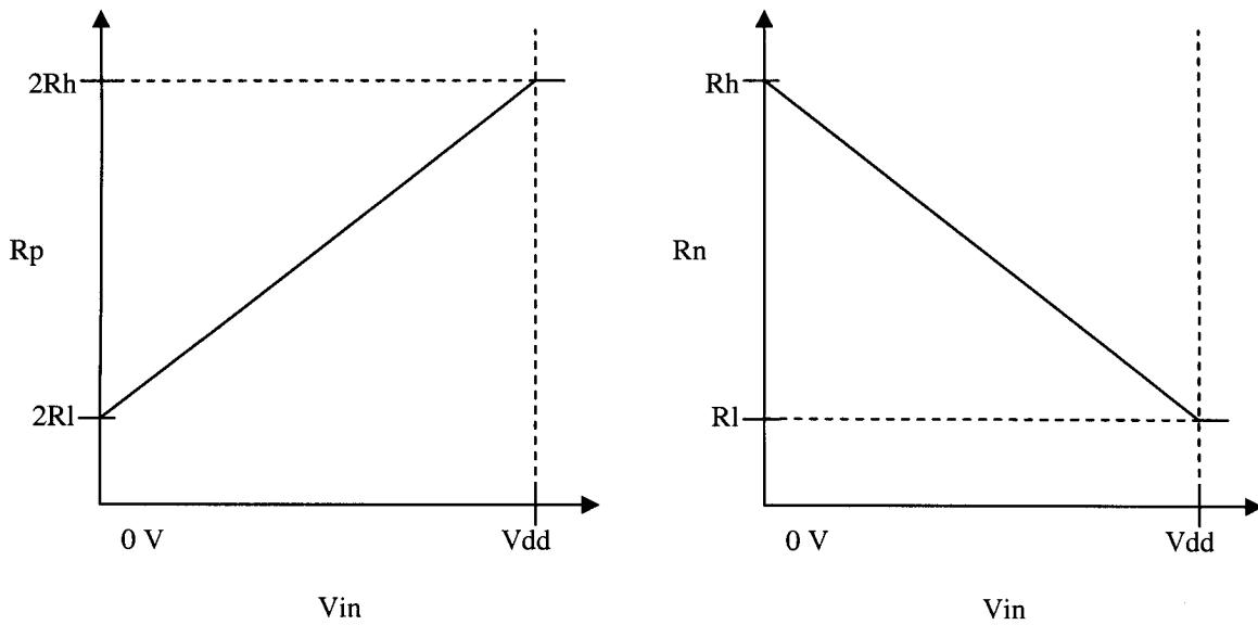
Derive equations for  $R_p$  and  $R_n$  in terms of  $V_{in}$ ,  $V_{dd}$ ,  $R_h$ , and  $R_l$ .
