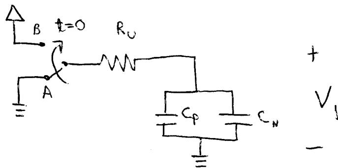
Solve your circuit for the input voltage,  $V_1$ , as a function of time. Use the constants  $V_{dd}$ ,  $R_u$ ,  $C_n$ , and  $C_p$  in your equation.
