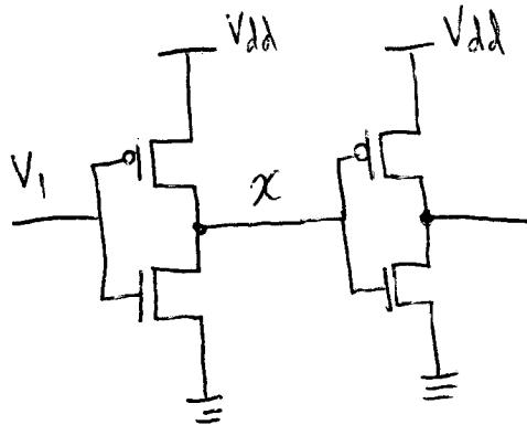
Replace the pFET transistors in the first inverter with resistors with resistance  $R_p$ . Replace the nFET transistors in the first inverter with resistors with resistance  $R_N$ . Finally, replace the pFET transistors in the second inverter with capacitances  $C_p$  and the nFET transistors in the second inverter with capacitances  $C_N$ . Draw the resulting circuit below.
