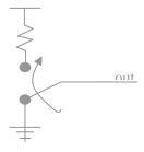
The "out" line could potentially be disconnected from both source and ground. In this case it is "floating."
