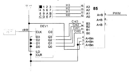
In the above schematic, clkM is the input master clock, DEV1 is the 4-bit counter, the LS85 chip is the comparator (with PWM output A>B) and a hex keyboard is used as the digital input. A switch is used to reset the counter's state.
