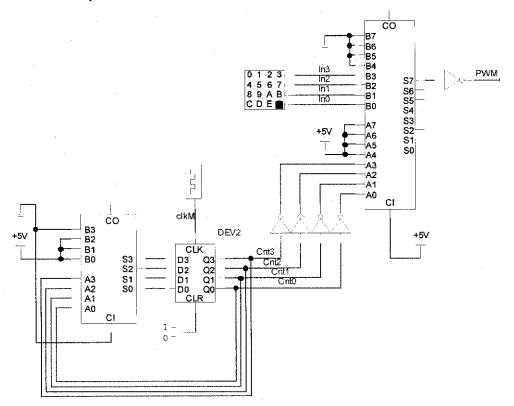
Here, a 4-bit adder, a 4-bit register (DEV2), and an 8-bit adder are used together to form the PWM output. As before, complete the following timing diagram for the above circuit:
