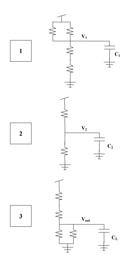
2.D. The above circuit requires 10 transistors but can be implemented with less. Design a transistor-level circuit that uses only 6 transistors to accomplish the same task.
