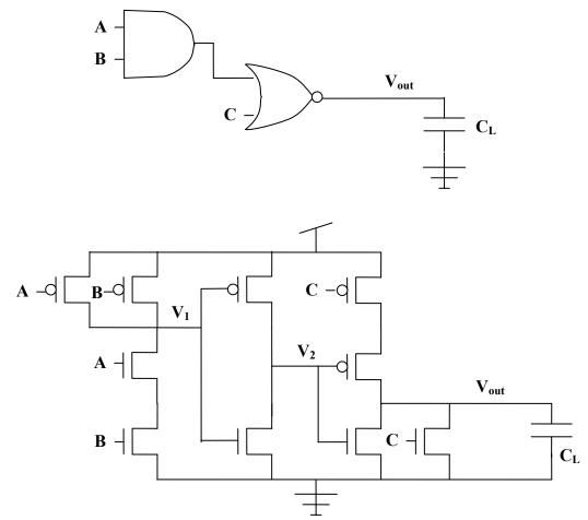
2.A. Divide the transistor circuit above into three sub-circuits (gates) and group these sub-circuits into two circuits corresponding to the two logical gates shown above. Clearly label each of the three sub-circuits, as well as the two larger circuits, with appropriate logical gate names.
